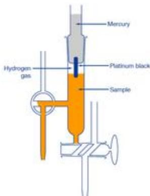
A hydrogen electrode is made by adding platinum black to platinum wire or a platinum plate. It is immersed in the test solution and an electric charge is applied to the solution and the solution is saturated with hydrogen gas. The electrode potential is measured between platinum black electrode and silver chloride electrode. This potential is inversely proportional to pH of the solution.
